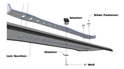
• Next take the bent Lexan brace and install it on the top section of the windshield. Remove the protective masking on both pieces prior to bolting the brace to the windshield. The bend will be above the bolts when installed. Please refer to the diagram below.
