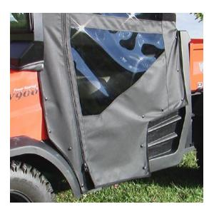
9. To open and stow the doors, move the zipper fully rearward and fold the bottom portion of the doors up. Then begin to form a vertical roll with the door by rolling it inward from the front edge toward the rear of the door. Secure in place using the two hook and loop straps provided. Try to form a roll approximately 2" in diameter to assure that the door will not stick out very far while stowed.
