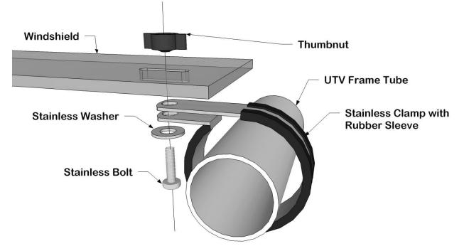
10. If using the Aero-Vent Lexan windshield with one of Falcon Ridge Cab Enclosures the top brace will be used to seal the top of the enclosure to the top of the windshield. After installing the enclosure over the windshield take a small knife and cut an x into the canvas where each hole is across the top of the windshield. Then install the brace as shown in the picture below.
