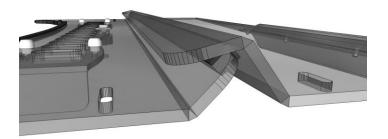
9. The diagram below shows the proper placement sequence of the hardware. Use the 1" bolts for this application. Install each one loosely at first; after you have centered the windshield and are satisfied with exact placement, then you may snug the thumbnuts appropriately.
