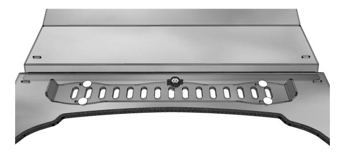
6. Next take the bent Lexan brace and install it on the top section of the windshield. Remove the protective masking on both pieces prior to bolting the brace to the windshield. The bend will be above the bolts when installed. Please refer to the diagram below.
