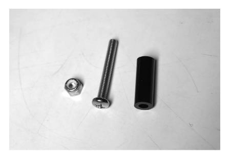
Take the spacer and slide it over the bolt as shown below
