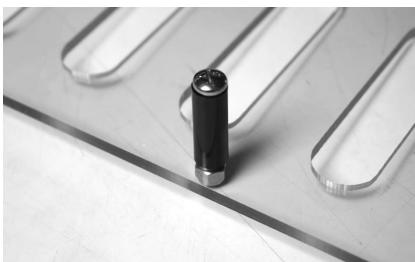
Now insert the bolt in the small holes and screw on the lock nuts so the end of the bolt is flush with the outside edge of the lock nut.
