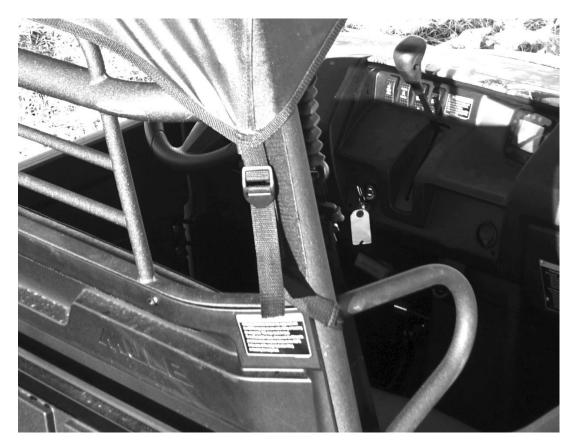
4. Once all the straps are in place run them through the buckles. Pull them tight making sure the top is centered and the side seams line up correctly along the roll cage. Once tight take a sharp knife or scissors and cut the straps so they are roughly 5-6" long, make sure to melt the ends to prevent fraying. The diagram below shows how to lace the webbing through the buckle.
