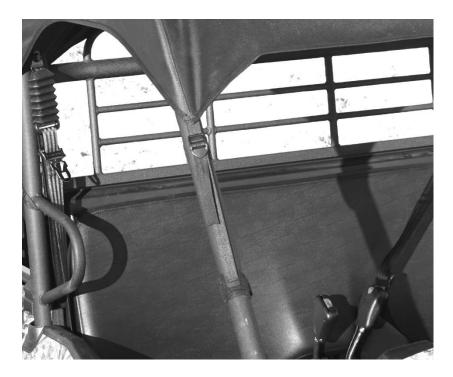
3. The rear of the Top Cap is held in place using the looped straps. This time wrap the loop around the roll cage so that it goes just under the side bars that help hold the passengers in place. Then take the other end of the strap and run it through the loop, pulling it tight. The photo below shows what it should look like.
