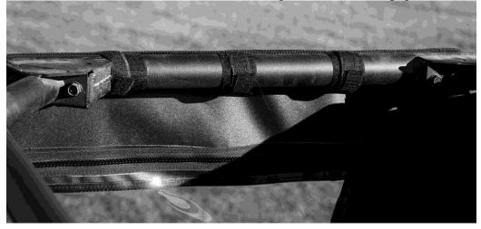
2. The rear edge of the doors has a strip of Velcro sewn down the entire length. This attaches to the Velcro sewn down the sides of the rear window. Magnets in the top rear corner hold it in place against the roll cage. See photos below.
