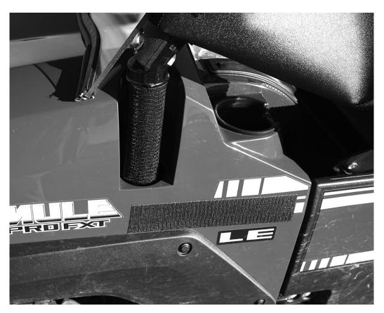
5. Finally, the bottom of the door has Velcro sewn across the entire length. Place the 25" adhesive Velcro strip on the outside of the door to match up with the bottom of the soft door. See photo below.
