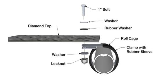
7. If you have a Falcon Ridge Windshield the two pieces are made to connect together using bolts. We suggest bolting the roof to the windshield before tightening down the clamps above. The photo below shows how the two pieces should be connected.
