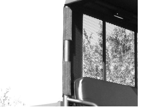
6. In the top corners, place a 3" adhesive strip on the inside of the bar where the double-sided Velcro strips are sewn perpendicular to the edges of the rear window. Photos below shows how this works.
