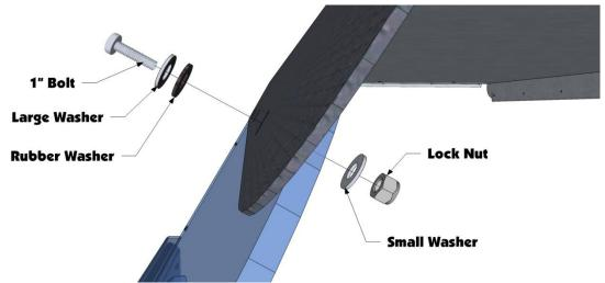
8. Make sure that the top and windshield are straight with each other. The bolt should fit in the middle of the slot on the roof. When together they should look like the photo below.
