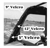
9. Along the top of the doors there are 5" and 6" Velcro loop tabs that should be attached as shown in the photo below.
