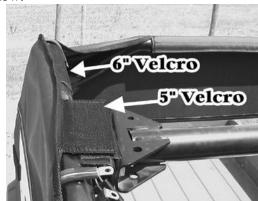
10. Next attach the supplied 10" and 5" adhesive Velcro strips the bottom of the floorboard and the rear of the cab as shown in the photos below.
