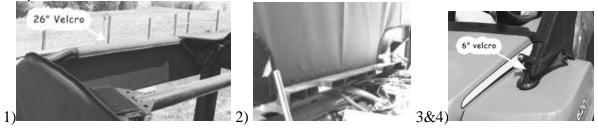
6. The two front pieces are attached by wrapping the 6" adhesive Velcro strip around the roll bar and then wrapping this with the double-sided strip attached to the enclosure. The photos below are an example:
