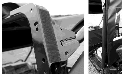
6. Now start at the bottom and attach the rear window making sure that it is centered. Then pull it up and attach the top and the sides last.
