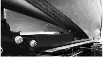
4. Next attach a piece of adhesive Velcro across the top bar, it should be placed on the top slightly angled towards the front of the vehicle. See Photo below.
