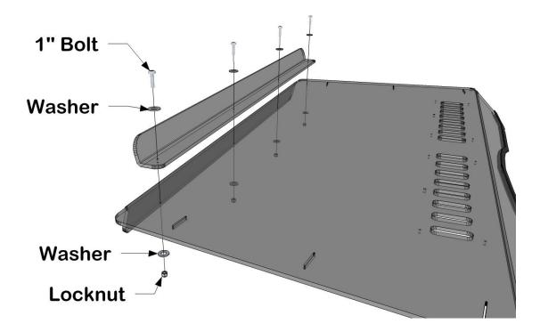
7. If you are using this windshield with a Falcon Ridge Cab enclosure, then you will use the Top Brace to sandwich the cab material and seal off the inside from the wind. The diagram below shows how it will work. If you aren't using one of Falcon Ridge Cab Enclosure you may opt not to use the Top Brace or install it for added strength.
