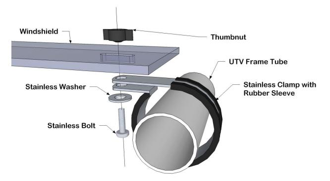
6. Now you can install the top brace if you want. If you do not have a Falcon Ridge Cab enclosure to work with this windshield, the top brace is not needed but can be installed for extra strength. Below is a diagram showing how the brace is to be installed.
