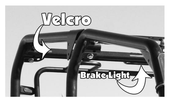
4. After placing the Velcro on the roll cage, attach the rear window. Across the top of the rear window is a cutout for the brake light, line this cutout up with the brake light and attach the rear window to the adhesive Velcro. See Photos Below:
