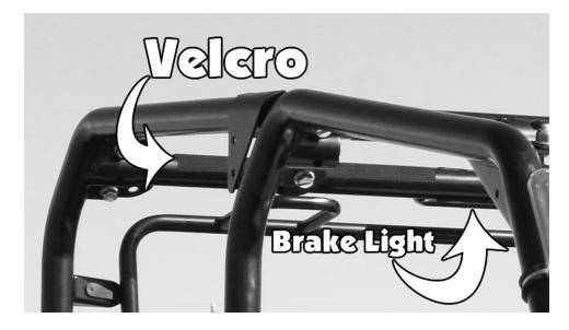
6. After placing the Velcro on the roll cage, attach the rear window. Across the top of the rear window is a cutout for the brake light, line this cutout up with the brake light and attach the rear window to the adhesive Velcro. See Photos Below:
