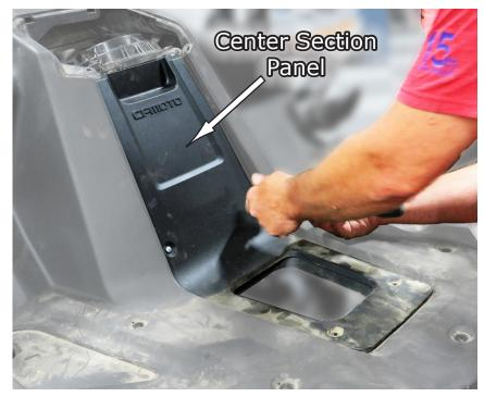
The center section will need to be removed before the main decking can be removed. So take this off first. See **Fig.31**.
