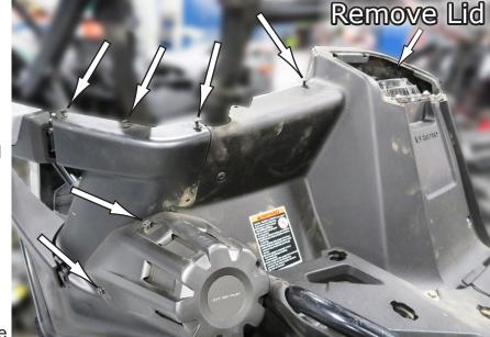
22. Then remove the three bolts holding the air filter on and remove the air filter. This will allow you to remove the cover it is attached to. See Fig.29.
