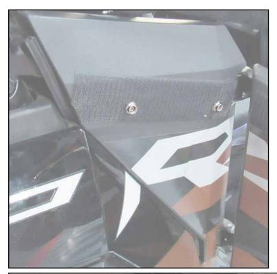
install Snap Studs to plastic with hardware shown
