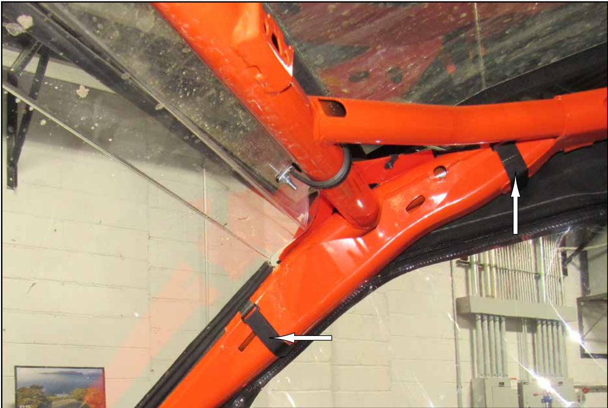
interior views of Straps secured to Frame
