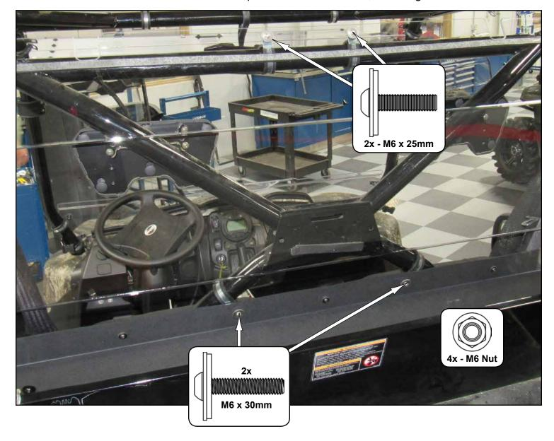
Align assembly to machine and tighten all hardware.
