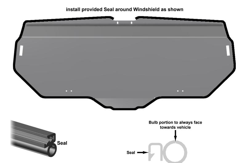
To ease installation, soak Seal in hot water before cutting or installing to increase flexibility.
