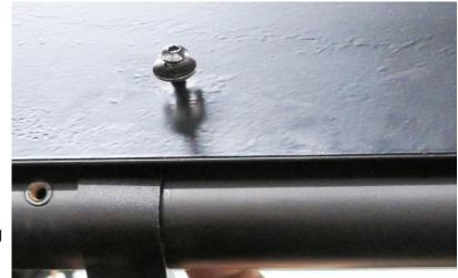
16. Next, install the roof to the clamps using the M6x20 Bolts with Sealing Washers, item "B" provided in your kit. You will use these for all 5 clamps. See Fig.13.
