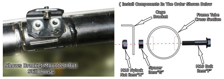
**21**. Once all the bolts, brackets, screws and clamps are all threaded and into place, make your final placement adjustment of the roof and tighten them all down securely.
