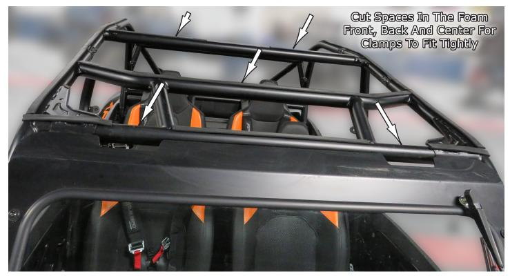
**11.** Now set the roof on the vehicle, See Fig.8. Next will need to install the rear corner bolts that attach the roof to the frame since these are in a fixed position. Then you can install the clamps and mounting brackets in the following steps.
