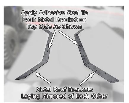
**4**. Now locate roof sections 1 & 2, and with using the two Roof Brackets, Sandwich the two Roof Sections with the Brackets as shown in **Fig.2**.
