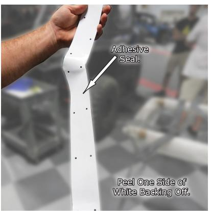
3. Then, peel one side of the paper off one of the Rubber seals and apply it to one of the Roof Brackets. Then peel and stick the other Rubber Seal to the other Roof Bracket, except make sure this bracket is mirrored opposite of the first one. Fig.1b shows both brackets laying opposite of each other and with the adhesive rubber seals already applied to one side of each metal bracket.
