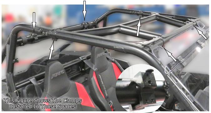
9. Next, install the clamps in the spaces you cut in the seal, but leave them a little loose so you can make final adjustments once all the clamps are installed and the top is placed on top. See **Fig.6**.
