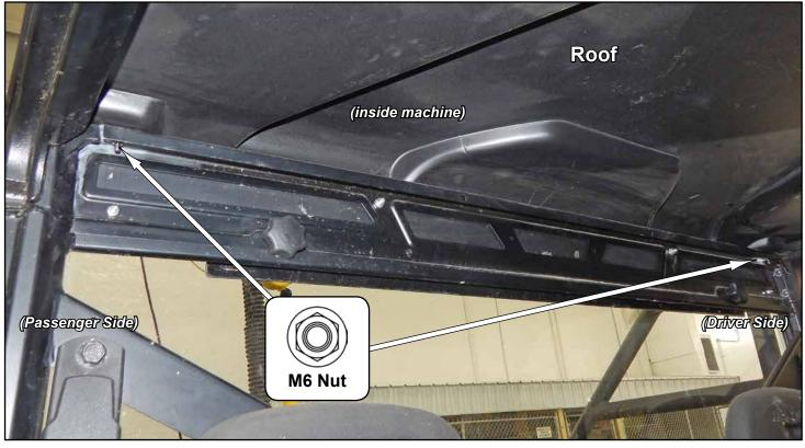
Align Roof to machine and tighten hardware completely
