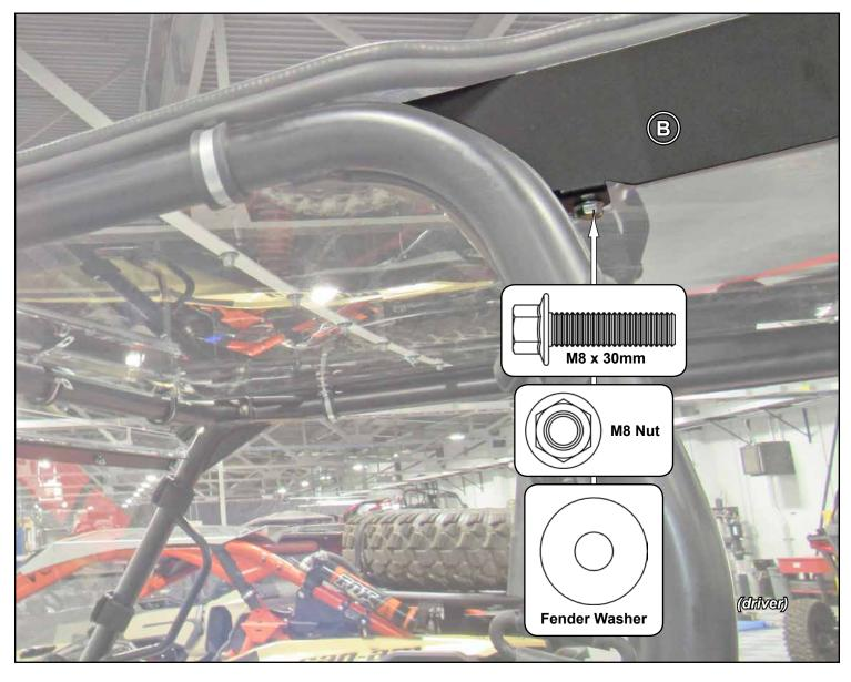
Align Roof to machine and tighten all hardware.
