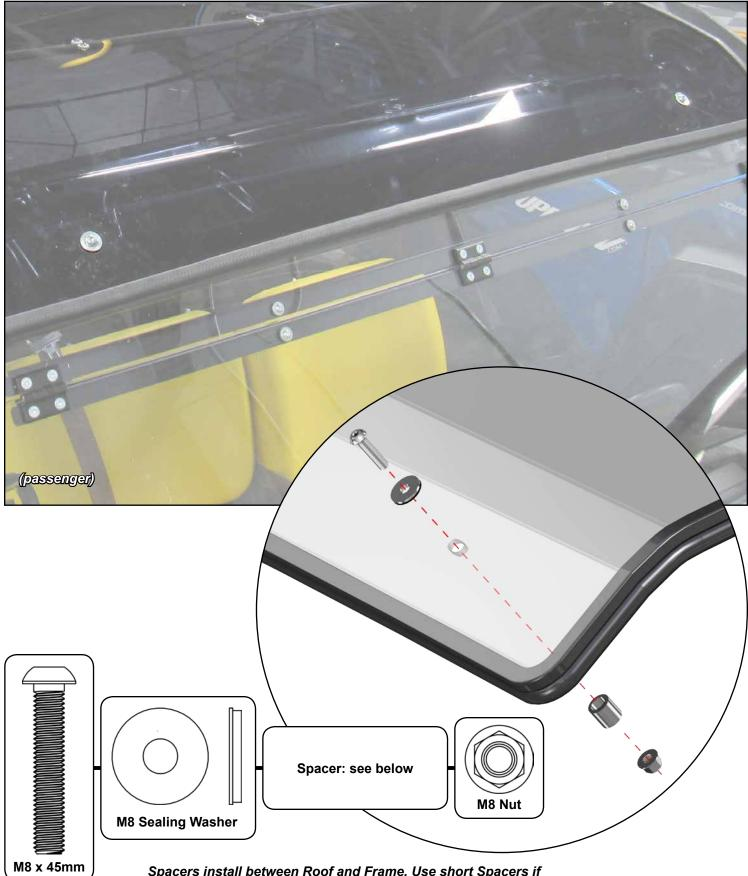
Spacers install between Roof and Frame. Use short Spacers if SuperATV Flip Windhield is installed. and long Spacers if not.
