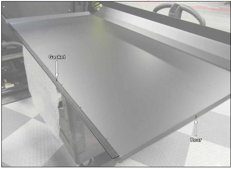
Install Gasket to Front. Gasket to run length of Front and cover mounting holes.
