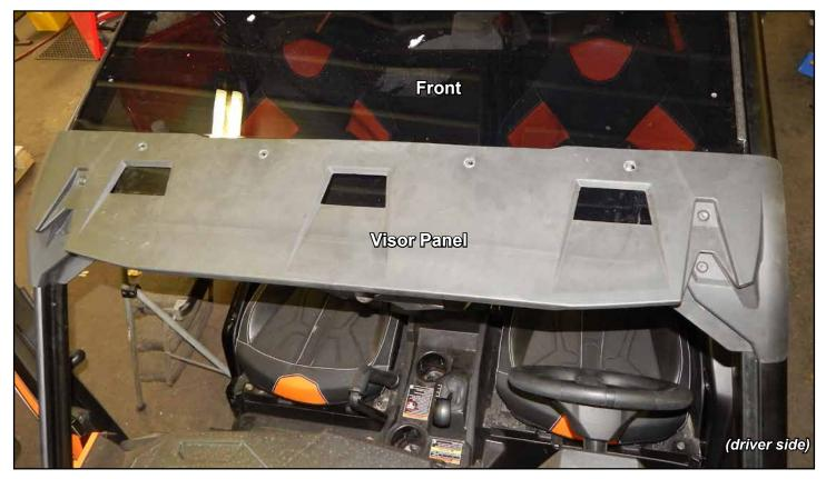
Align Roof to machine and tighten all hardware completely
