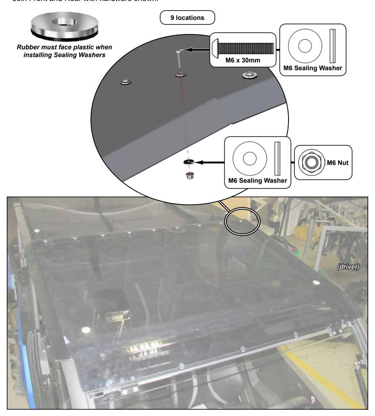
align Roof to machine and tighten all hardware completely
