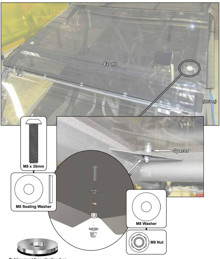
Rubber must face plastic when installing Sealing Washers
