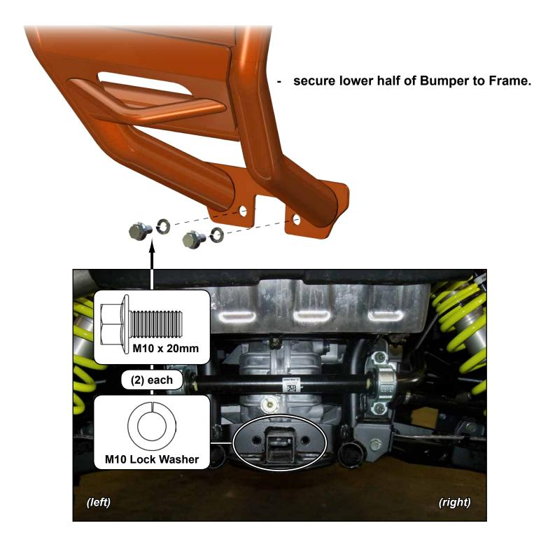
Align to machine and tighten hardware completely.
