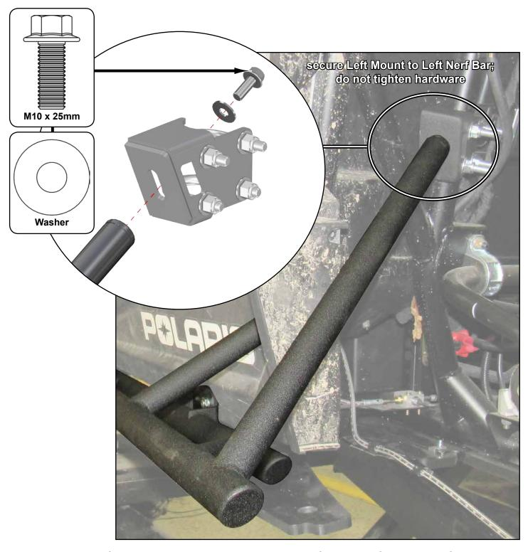
align Nerf Bar to machine and tighten hardware from rear of machine to front
