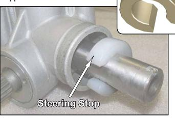
Leave Boots off Rack and Pinion until new Tie Rods are installed.
