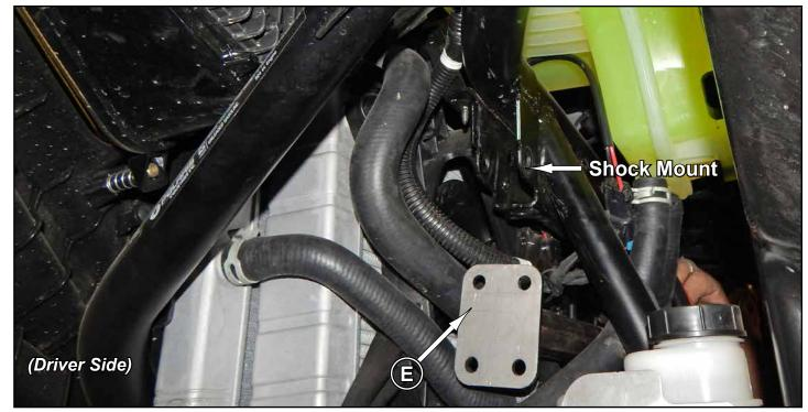
Secure Left Front Bracket (B) to Cross Brace (E) with hardware shown.
