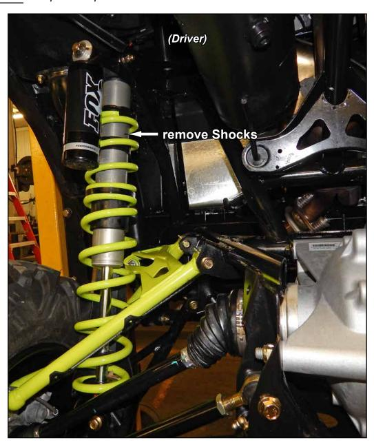
SuperATV highly recommends using a Spring Compressor when removing Springs
