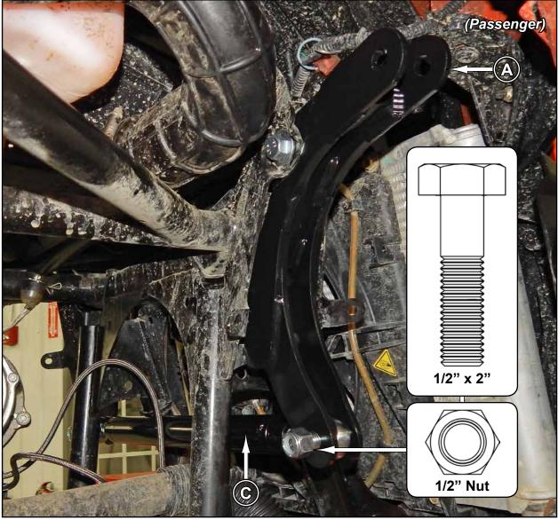
Tighten hardware completely.
