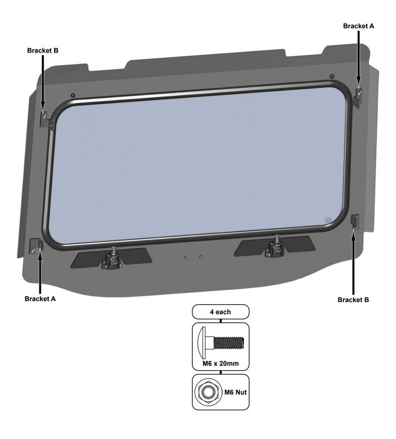
Secure Clamps to Cage in locations shown with previously removed hardware; do not tighten completely.
