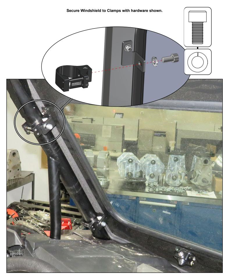
Align assembly to machine and tighten all hardware.
