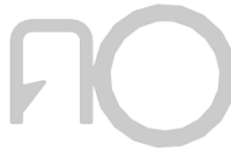
Bulb portion of Seal to face towards vehicle
