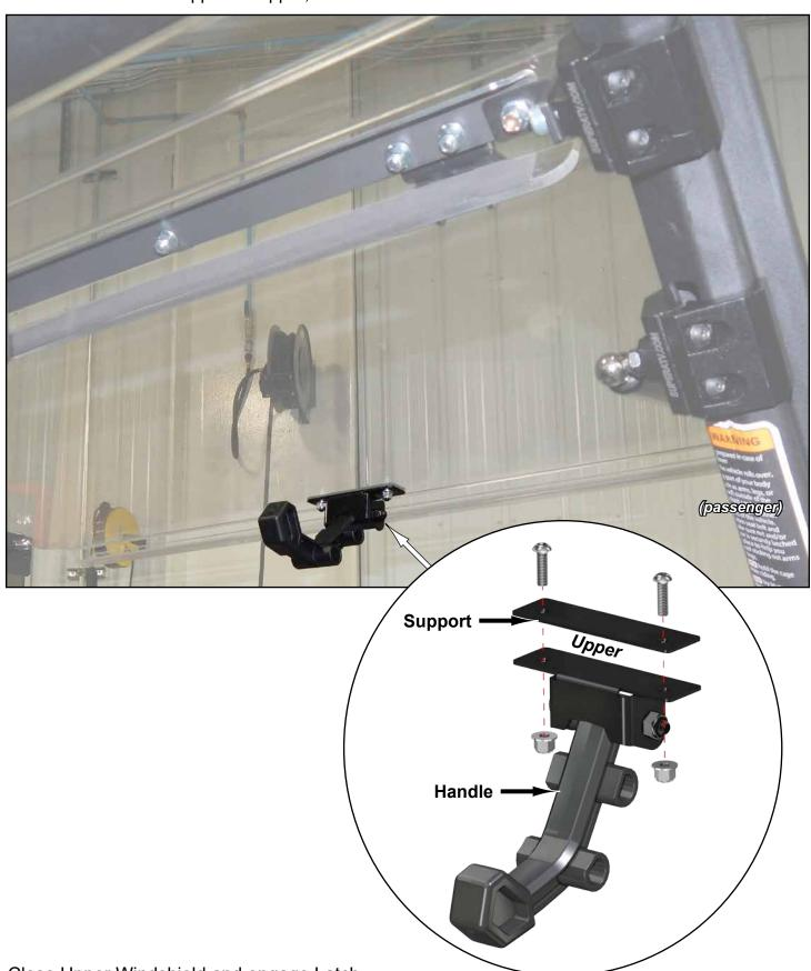
Close Upper Windshield and engage Latch.Align Windshield assembly to machine.
