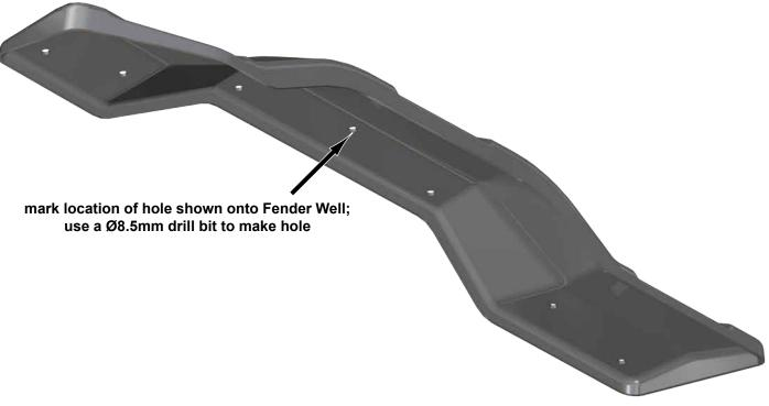
secure Upper Right Rear Fender Flare with provided Push Pin
