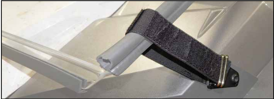
- Pull Strap tight and secure.
