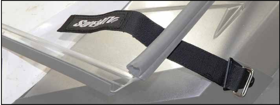
- Loop Strap around Windshield and through Strap.
