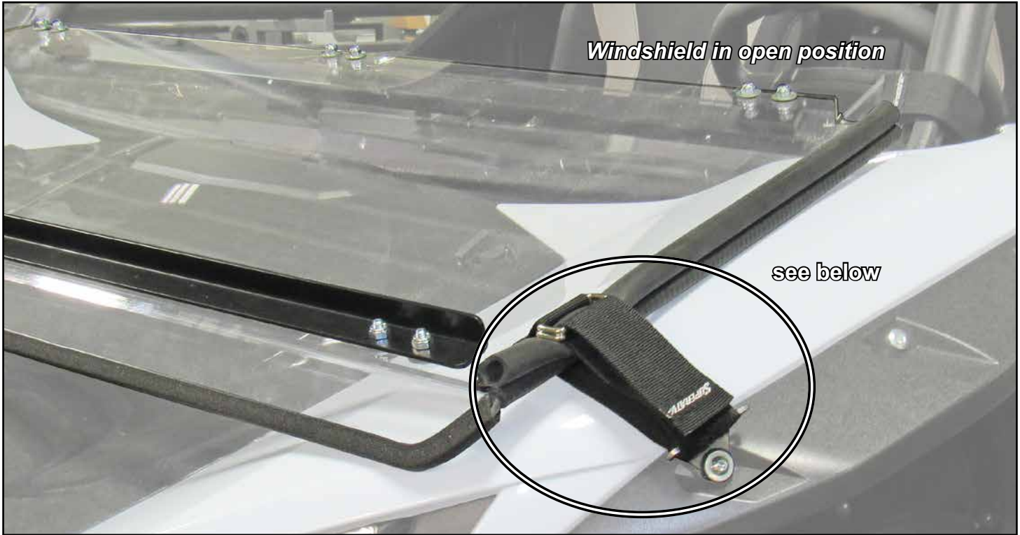
- Loop Strap through Windshield and Strap.
