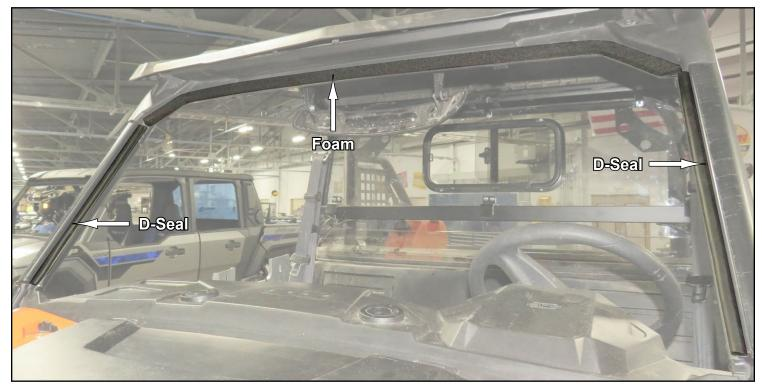
Install Seal to Lower Mount in location shown.
