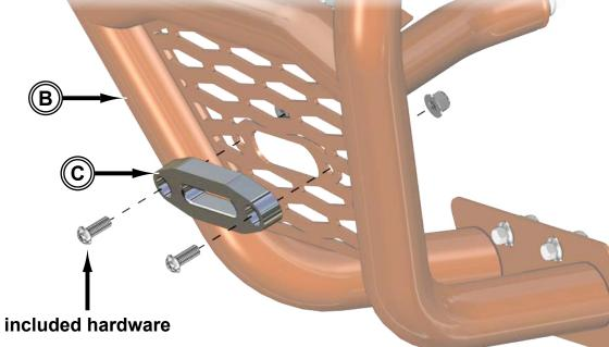
Tighten all Lower (B) hardware and reinstall Grille before installing Upper (A).
