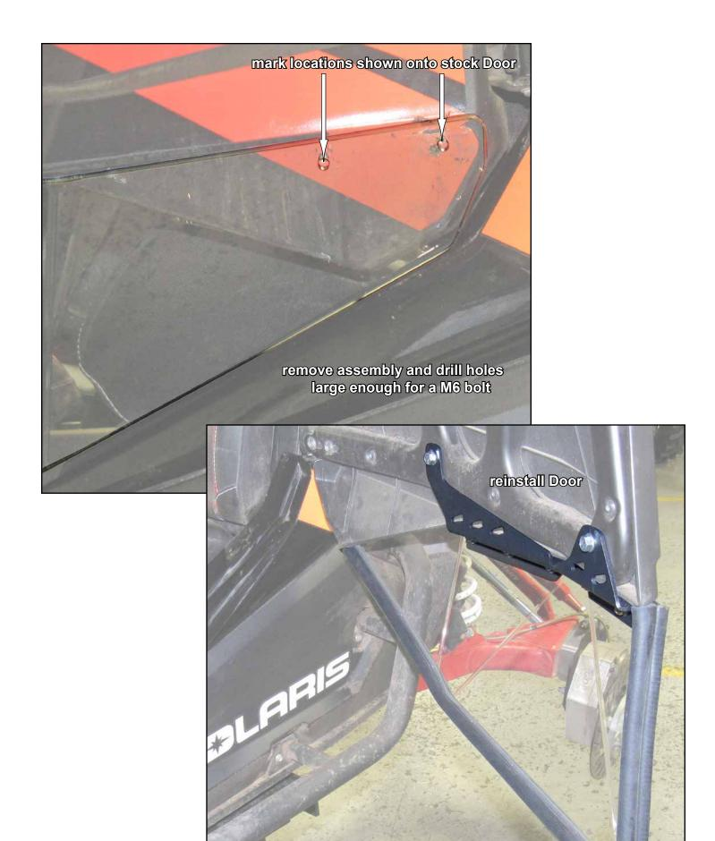
2 each - Secure Left Insert (B) to stock Door with hardware shown; tighten completely. M6x 25mm **Sealing Washer** M6 Nut
