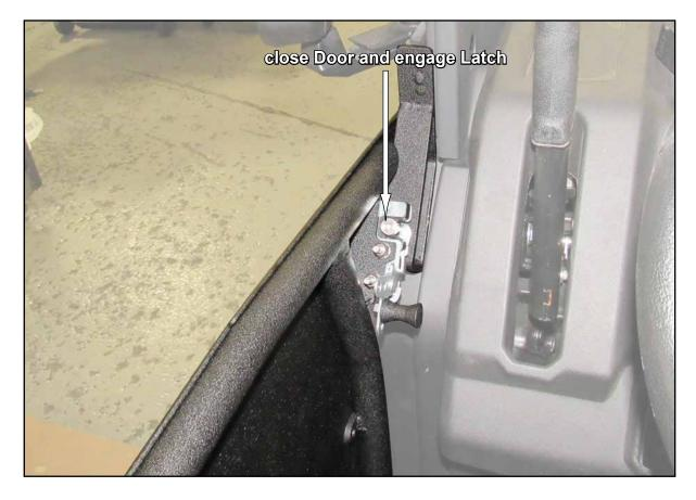
align Door to machine and tighten all hardware completely
