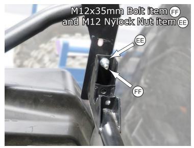
Now that the top bolts are in place, attach the Pivot Tube Assy to the Lower Holes using the M12x35 Hex Bolt, item (FF). Tube Mount Assy is tapped for this bolt, so no Nut is required.
