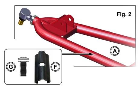
Secure Brake Lines to A-Arms (A-B) with Brake Line Clips (F) and M5-.8 x 13mm Lg. PHMS (G).
