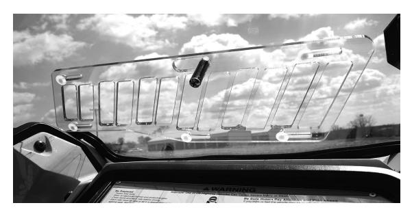
6. You are now ready to install the windshield on your roll cage. Place the windshield on the vehicle first. Begin with the Bolts in the top corners of the windshield. Using a 1" bolt two washers and a lock nut fasten them as shown in the photo on the next page.
