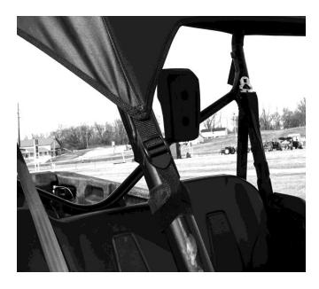
4. Next take the other two straps with loop sewn on one end and wrap them around the roll cage on the cross bar. See photo below.
