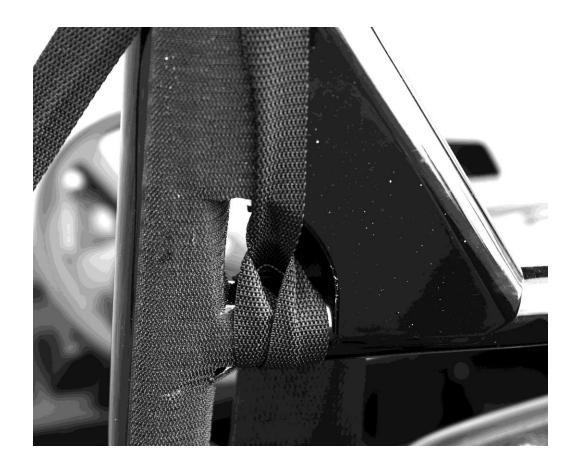
5. Now place the top over the entire vehicle, the front of the top is identified by the sides being more steeply curved, and begin by lacing the front straps through the ladder lock buckles sewn to the front corners of the top. Diagram below shows how to use ladder buckle.
