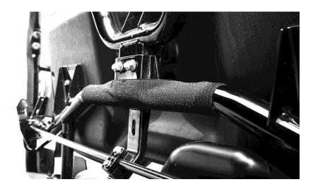
**6.** After attaching the top and bottom attach the two 32" adhesive Velcro strips to match up with the sides of the Rear Window. Starting just below the top cross bar place the 32" adhesive strips down the bar facing the rear of the vehicle. Then pull sides of the Rear Window and attach them down the bar to the Velcro. See Photo below.
