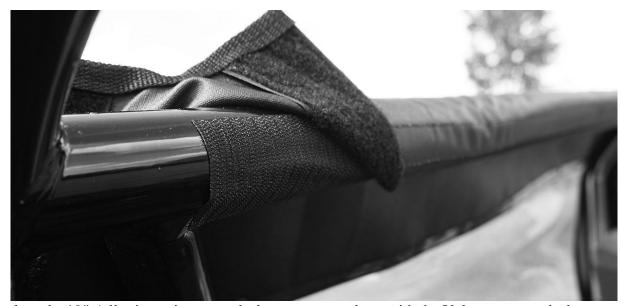
5. Next place the 19" Adhesive strip across the bottom to match up with the Velcro sewn to the bottom of the Rear Window. See photo on next page.
