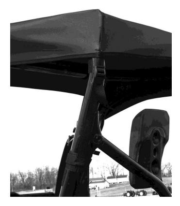
5. Now place the top over the entire vehicle, the front of the top is identified by the sides being more steeply curved, and begin by lacing the front straps through the ladder lock buckles sewn to the front corners of the top. Diagram below shows how to use ladder buckle.
