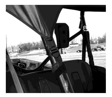
4. Next take the other two straps with Velcro sewn on one end and wrap them around the roll cage in the rear about 10-12" below the Top Cap. Be sure to wrap the 6" adhesive strip completely around the bar and then tightly wrap the double-sided Velcro around the adhesive strip. See photo below.
