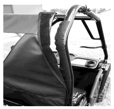
**12.** Now just hang the rear window from the Velcro on the top bar and attach it down the sides. The bottom of the rear window has magnets that will attach to the frame.
