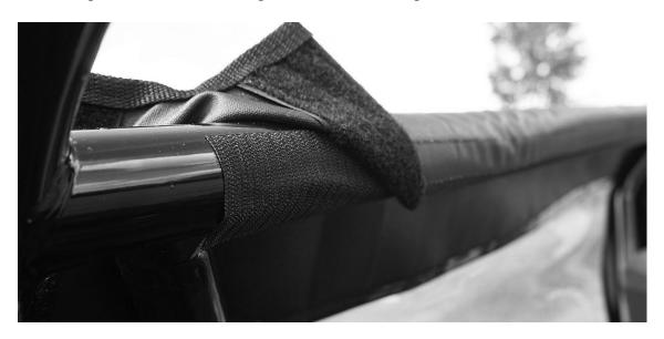
11. Next attach the sides to the double-sided velcro tabs sewn along the rear of the doors as shown in the photo on the next page.
