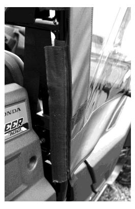
**6.** Now move to the front lower corner and place the 9" adhesive strip to match up with the Velcro on the cab. See photo on next page.
