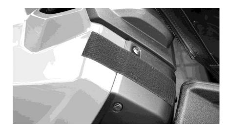
7. Last Item on the doors will be a snap on the inside front section of the plastic doors. Its easier to place the snap in the right position by first putting the screw snap stud into the socket on the enclosure. Then pull the door into place and push the snap into the plastic so that an mark is left. Then pull the snap out and screw it into the door making sure not to over tighten and strip out the plastic. See Photos Below.
