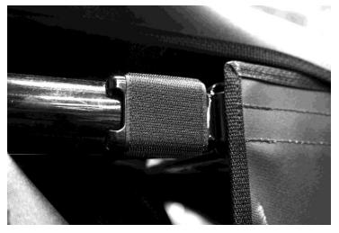
9. Then take the Rear Door and zip it to the Middle Rear Window. This ensures the door is properly placed. Then attach the top front corner to the Velcro. See photo below.
