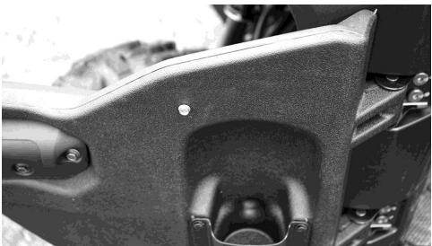
8. Begin by placing the 4" adhesive Velcro strip in the top front corner on the flat surface shown in the photo below.
