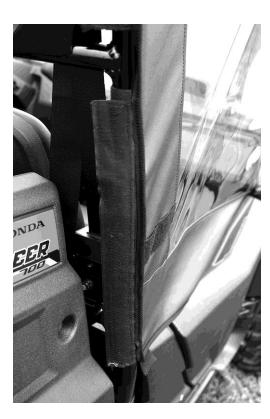
**6.** Now move to the front lower corner and place the 9" adhesive strip to match up with the Velcro on the cab. See Photo Below.
