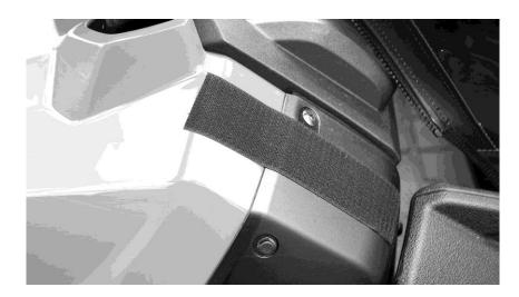
7. Last Item on the doors will be a snap on the inside front section of the plastic doors. Its easier to place the snap in the right position by first putting the screw snap stud into the socket on the enclosure. Then pull the door into place and push the snap into the plastic so that a mark is left. Then pull the snap out and screw it into the door making sure not to over tighten and strip out the plastic. See Photos Below.
