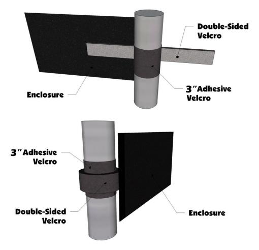
5. After attaching the double-sided strips go to the rear of the door. You will see three Velcro tabs sewn here. Starting just below the top cross bar place the 32" adhesive strips down the bar facing the rear of the vehicle. Then pull the tabs around and attach then down the bar to the Velcro. See Photos below.
